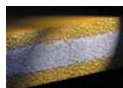
Cross section of Infinity's patented ceramic/metal matrix. Outer layers are pure alumina, deep-etched to an internal aluminum substrate.
